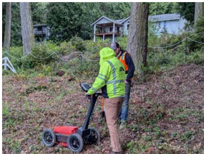
Contractor conducting Ground Penetrating Radar Survey at Port Ludlow Cemetery.
